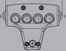
Edition: Sensor installed Pos. 5, Push button installed Pos. 1,2
