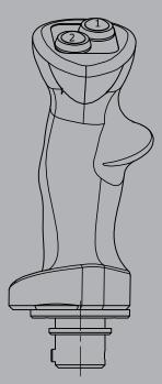
**B15**Push button installed Pos. 1,2
