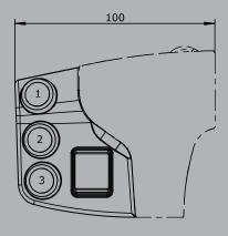
Edition installed right: Push button installed Pos. 4,5,6 Rocker switch
