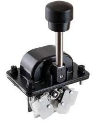
Example S23L S5 М - 3 Z P - A050 P134 - X Basic unit S23L left Control-handle extended -20 mm Grip / palm grip Mechanical zero interlock Axis 1 (direction 1-2) 3 3 contacts (2A 250 V AC15) Z Spring return Р Potentiometer Description axis 1 (direction 1-2) A050 Arrangement MSP21-0 P134 Potentiometer T396 2 x 5 kOhm Special model Special / customer specified
