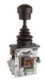
Example S22L S5 т - 3 Z P - A050 P134 - X Basic unit S22L left Control-handle extended -20 mm Grip / palm grip Dead man Axis 1 (direction 1-2) 3 3 contacts (2A 250 V AC15) Z Spring return Р Potentiometer Description axis 1 (direction 1-2) A050 Arrangement MSP21-0 P134 Potentiometer T396 2 x 5 kOhm Special model Special / customer specified
